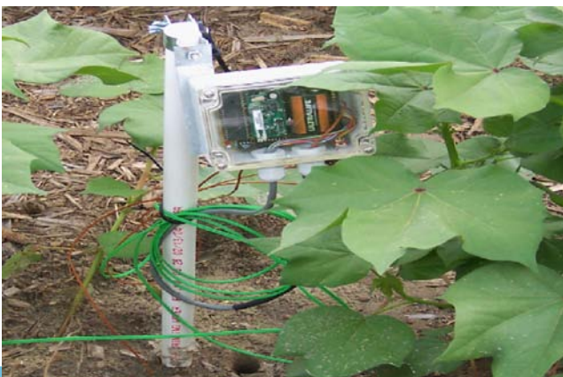
Figure 1 Schedule irrigation in cotton farm using RFID and sensor
